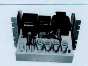
The 200-watt Power Amplifier is a bridging type amplifier using four Type 6550 beam tetrodes in a push-pull, Class AB<sub>1</sub>, circuit. Its exceptional frequency response and low distortion make it ideal for wide-range reproduction of music. When more than one amplifier is used in a system the inputs are paralleled. With 16 decibels of inverse feedback for frequency stabilization, it produces 200 watts of clean audio power.
