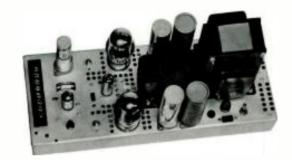
The Type SA-1000 is a compact, tube-powered 100-watt amplifier for use wherever high quality and long life are appropriate. It provides an unbalanced bridging input and a multi-impedance output. The input is convertible to balanced with an optional transformer (see Accessories).
