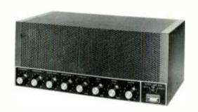
The Type SA-1004 is essentially an extension of the Type SA-1000 described above with four microphone preamps, two auxiliary inputs (for high-level phono or tuner) in addition to bridging input. Separate bass and treble tone controls are also included. The bass control cuts 20 and boosts 15 dB at 50 Hz; the treble control boosts 10 and cuts 20 dB at 20 kHz.
