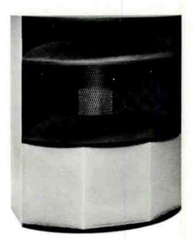
The LC-9 Loudspeaker System is designed for applications where high acoustical level, wide dispersion angle, and extended frequency response are required. The frequency range is covered by separate low and high frequency horns with a crossover point at 500 Hz. A feature of the LC-9 is the particular care with which the high and low frequency horns have been designed to provide matched acoustical wavefronts for smooth response over the entire frequency range.
